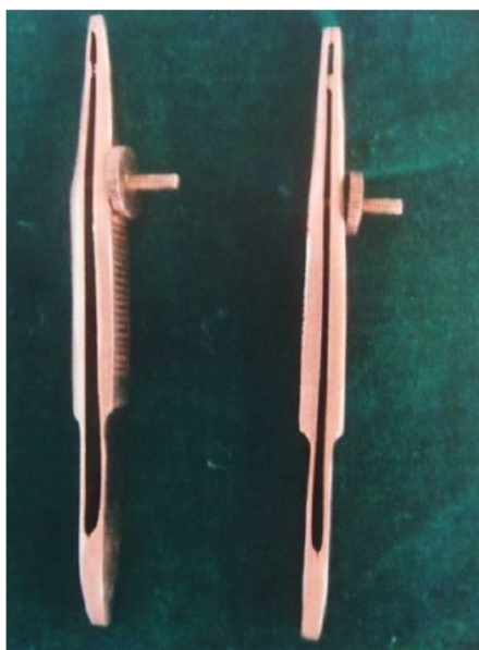
Figure 6: - Custom made stainless steel testing forceps
