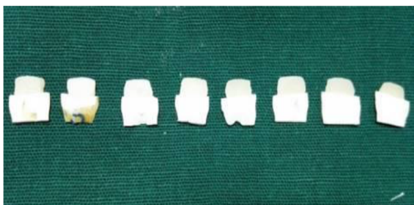
Figure 5: - Beams obtained after sectioning of samples
