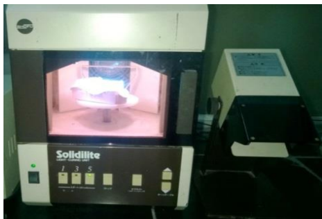
Figure 4: - Curing Inside Curing Chamber (Solidite Shofu)
