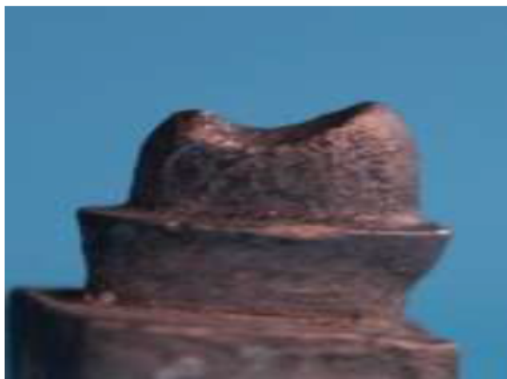
Figure 1: Master metal die with 8° taper
