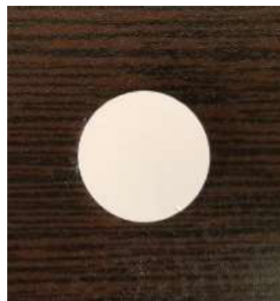
Figure 1: Sinter less cut out zirconia sample from the main block
