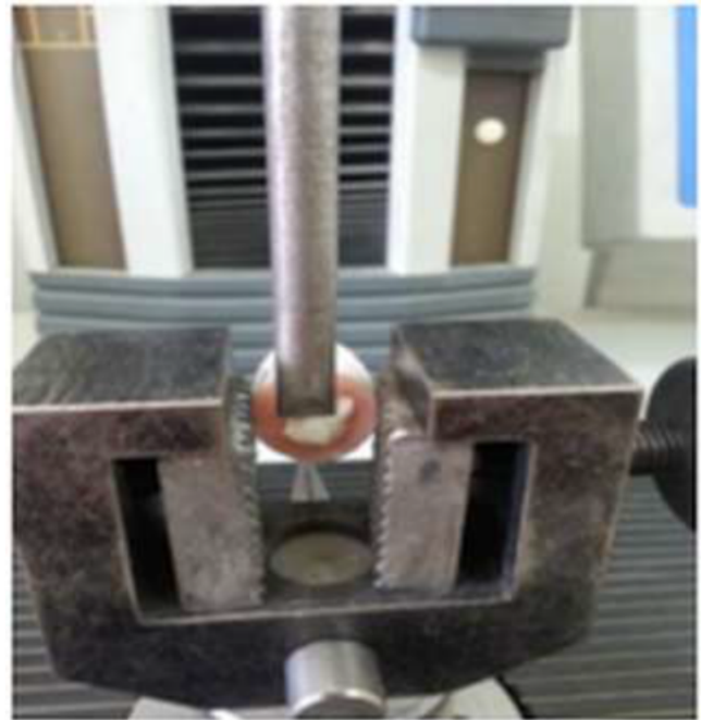
Figure 1: Specimens mounted on the universal testing machine for the measurement of shear bond strength
