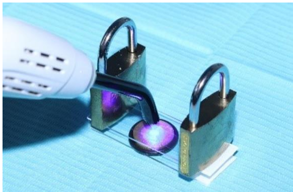
Figure 1. Construction of discs specimens
