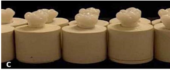
c) Figure 3. Resin test blocks: a) Resin test blocks with embedded duplicate abutment teeth. b) Digital scan and design of the tested PICN hybrid ceramic crown. c) Resin test blocks with cemented crowns.
